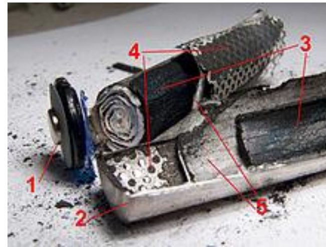
Figure 3-3: Cross-section of a prismatic cell.
